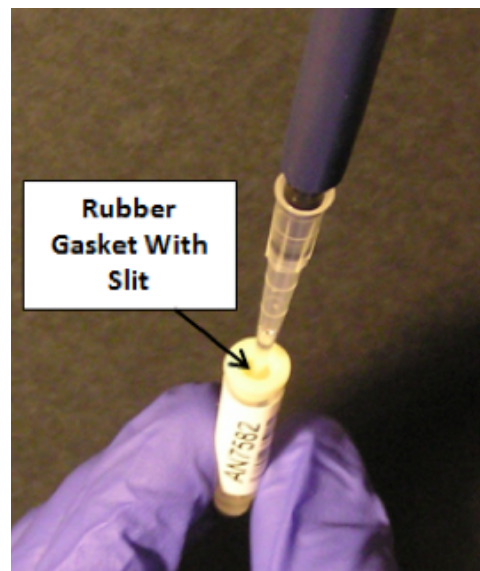
Figure 4.3: Pipetting the Sample into the Operon Sequencing Tube by Gently Forcing the Pipette Tip through the Gasket.
