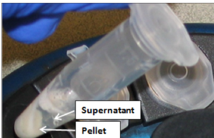
Figure 1.2: Spinning the Microfuge Tube Separates the Supernatant From the Pellet.
